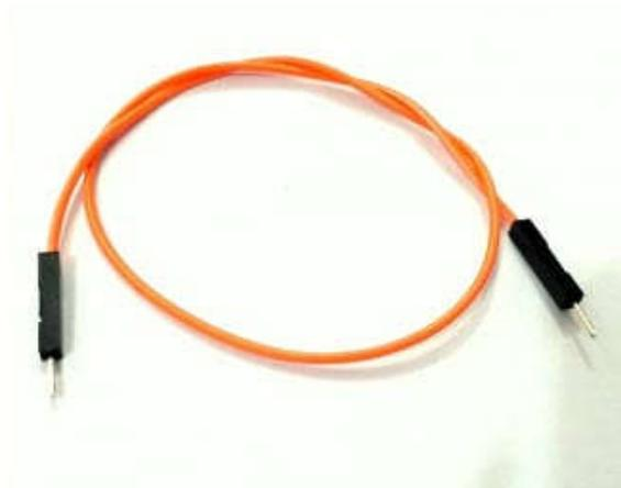
Gambar 2.9 Kabel Jumper Male to Male
