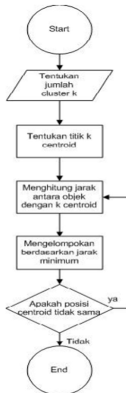
Gambar 2. 2 Flowchart Algoritma K-Means
